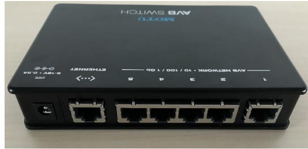
Abb. 42 – MOTU AVB-Switch Anschlüsse
