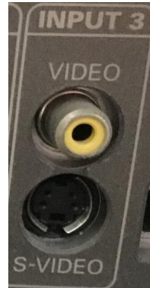
Abb. 77 – Composite- (oben) & S-Video (unten)
