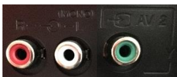
Abb. 90 – Composite-Video inkl. Stereoton-Anschlüssen
